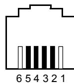
Figure 4 : RJ11/12 socket, front view
